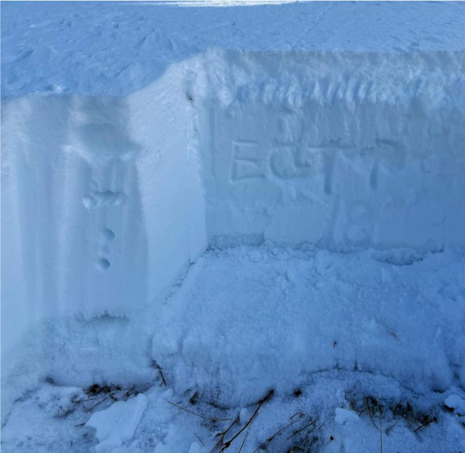
Snowpit and ECT result from small slope just above Beehive Creek at 8200 ft.
