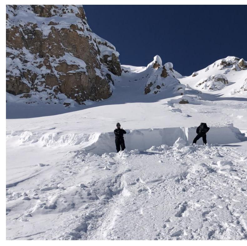
We dug in 1 crown and measured 11" of SWE above the weak layer (1mm facets) that avalanched. Every weak layer has a breaking point, and this layer needed about 11 feet of snowfall to get it to avalanche.
